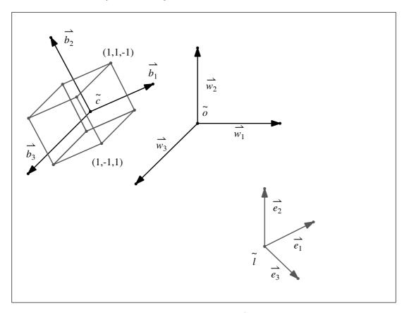
In the diagram above, we are positioning ourselves at a location l in the world coordinate system, and we are looking in the direction of the negative of the basis vector  $\vec{e_3}$ . The other two basis vectors in the eye coordinate system orient us in space: in particular, the basis vector  $\vec{e_2}$  establishes our *up direction*.
