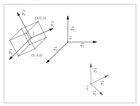
Rightward from our perspective is in the direction of the vector  $\vec{e_1}$ . Unfortunately, this does not line up with the object's interpretation of rightward, which runs in the direction of  $\vec{b_1}$ . If we wanted the object to move, say, one unit to the right relative to its own coordinate system, we could just apply the transformation
