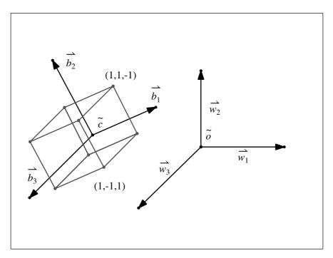
In the diagram shown here, one of the vertices that makes up the cube has coordinates (1,1-1) in the object coordinate system with basis  $\vec{b_1}$ ,  $\vec{b_2}$ , and  $\vec{b_3}$ . Ultimately, we will want to know what that vertex location is in world coordinates. This can be determined by setting up a transformation matrix that transforms the world frame to the object's coordinate frame. In homogeneous coordinates, that transformation matrix is
