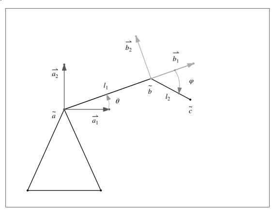
The coordinate frame positioned at  $\tilde{a}$  acts as the object coordinate frame for the entire model. The robot has joints at  $\tilde{a}$  and  $\tilde{b}$  that can be rotated independently: the diagram shows the joint at  $\tilde{a}$  rotated through a positive angle  $\theta$  and the joint at  $\tilde{b}$  rotated through a negative angle  $\varphi$ .
