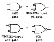
Fig. 3. Functional equalities of pairs of gates.
