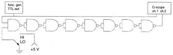
Fig. 6: Circuit for measuring TTL gate response by method I.
