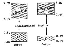
Fig. 1. Voltage ranges for TTL.
