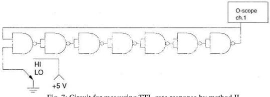
Fig. 7: Circuit for measuring TTL gate response by method II.
